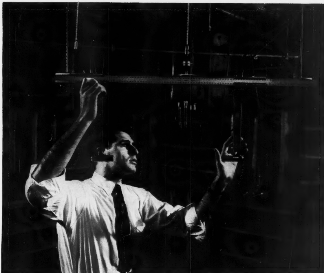
In a quiet room at Bell Laboratories an engineer scales off the distance between two condenser microphones during a calibrating test. Able to measure air pressure variations of a few billionths of an atmosphere, such microphones play a crucial role in the scientific study of telephone instruments.
